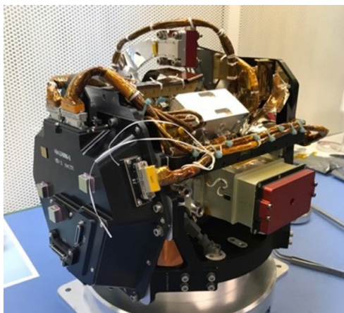
Figure 1. The completed MAIA camera assembly.
